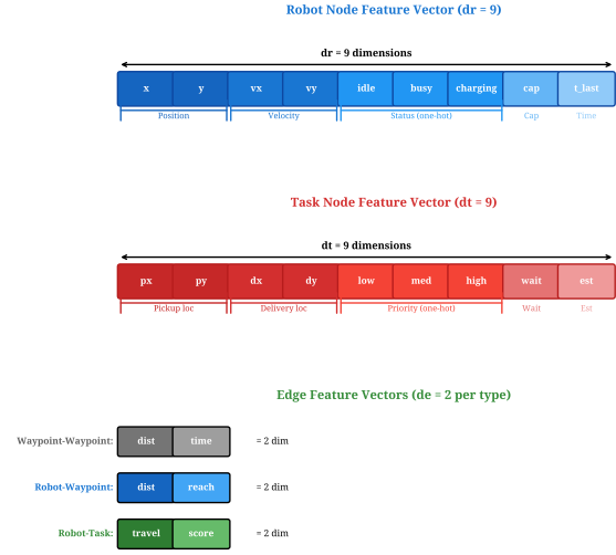
Fig. 2. Visualization of node and edge feature vectors. Feature vectors for robot, task, and edge types and their dimensions.
